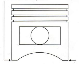
\*NOTE: IF PISTONS ARE PRO-COATED, SUBTRACT .002 FROM CLEARANCE NUMBER.
